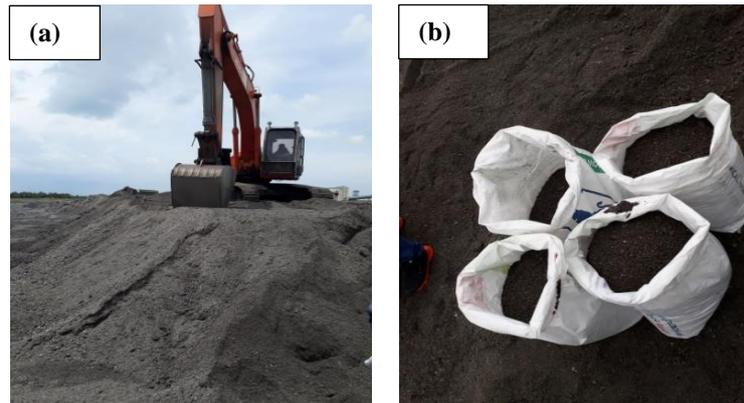
Fig. 2 - (a) Fresh bottom ash deposited at power station, (b) Collected bottom ash for the study
