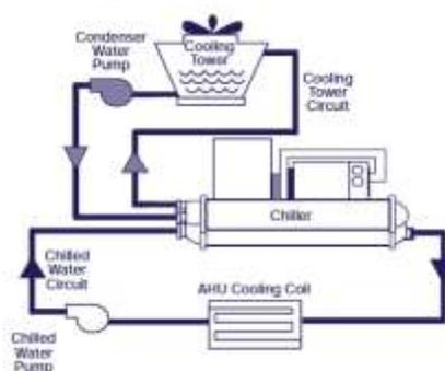
Fig. 3 - Typical water-cooled chiller system (adapted from energy-models)
