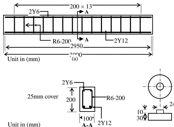
Fig.4. Reinforcement and projectile details
