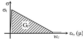
Fig.2. Strain-softening in tension
