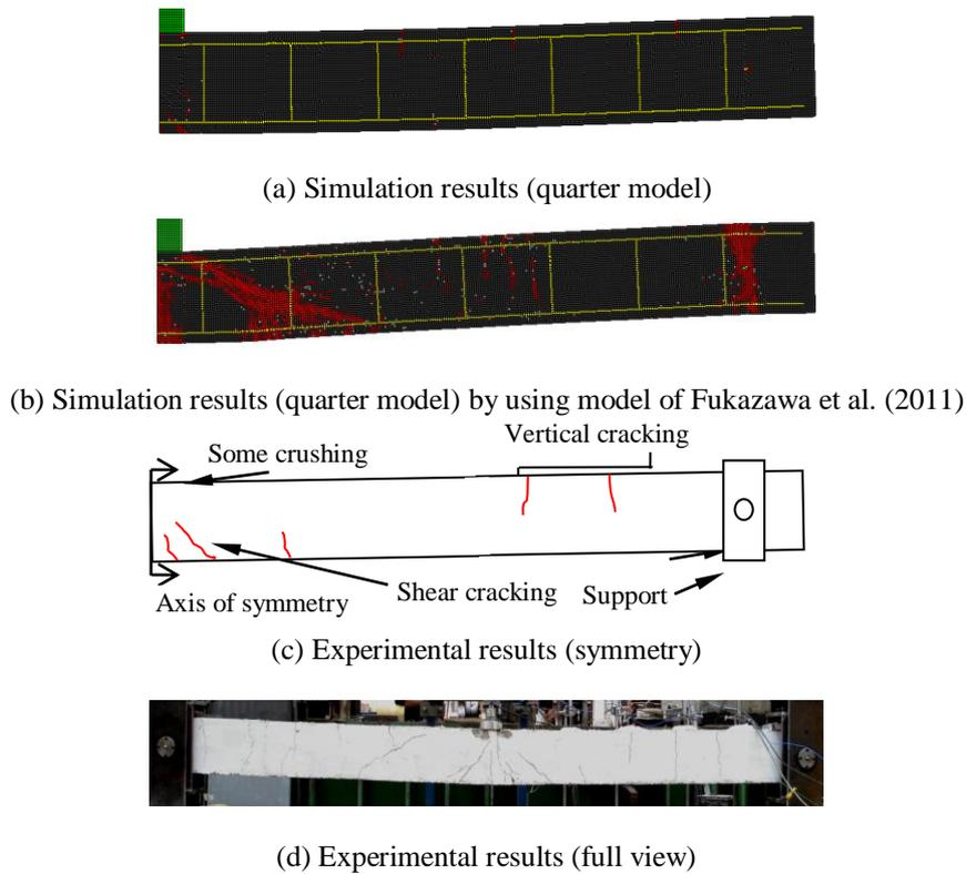
Fig. 6. Comparisons of pin-ended support beam between numerical with experimental results
