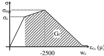
Fig.3. Hardening and strain-softening in compression
