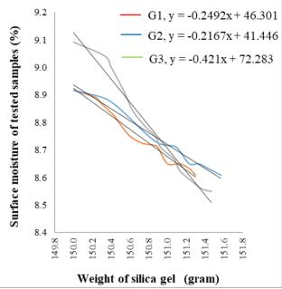
Fig. 8 - Relationship between average surface moisture content of mortar with weight of silica gel
