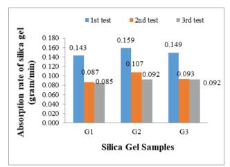
Fig. 7 - Absorption rate of silica gel for each mortar sample
