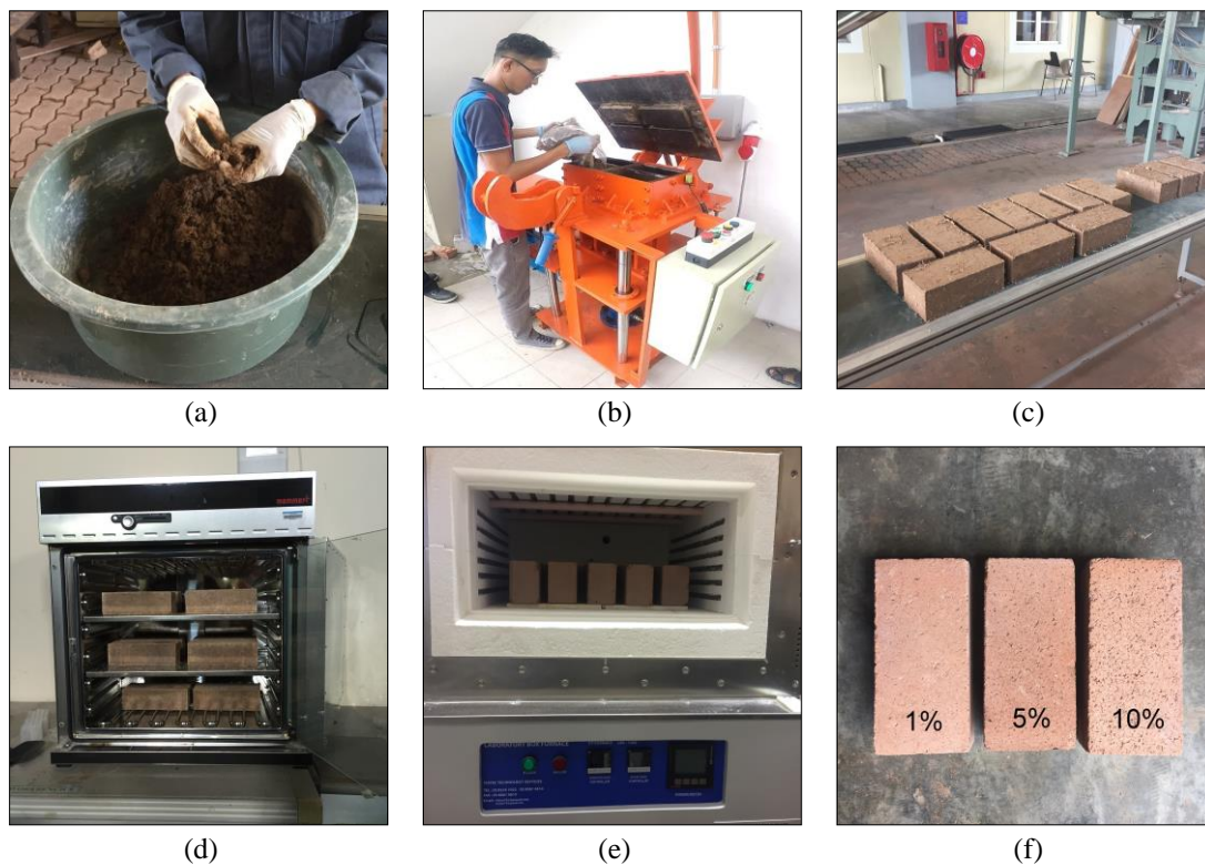
Fig. 2 - (a) Mixing soil and POFA with predetermined water; (b) Compress in brick machine; (c) Drying at room temperature; (d) Drying in ventilated oven; (e) Firing in laboratory furnace; (f) POFAB after firing
