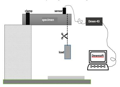
Fig. 11 - Experimental set-up of simple laboratory
