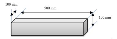
Fig. 10 - The beam specimen of mortar or concrete
