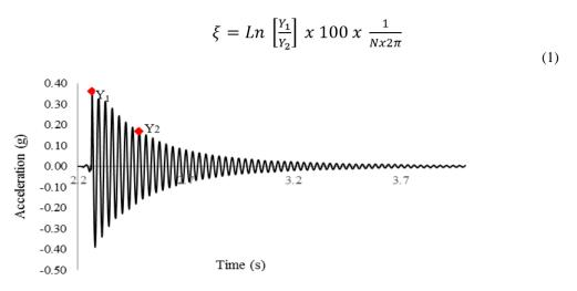
Fig. 12 - The logarithmic decrement signal at the free end of the beam
