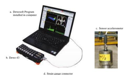
Fig. 8 - A unit dynamic laboratory equipment
