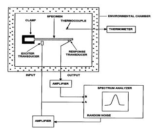
Fig. 2 - Experimental set-up of ASTM E756-05 method
