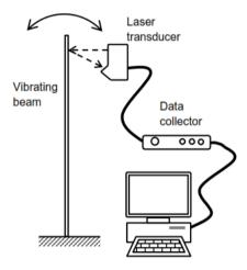
Fig. 6 - Experimental Set-up of Pérez-Peña et al. (2016)
