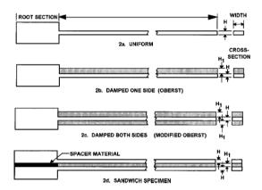
Fig. 1 - Test Specimen of ASTM E756-05 Testing
