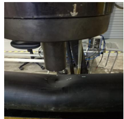
Fig. 10 - Elastic Rebound of RTP after process of unloading.
