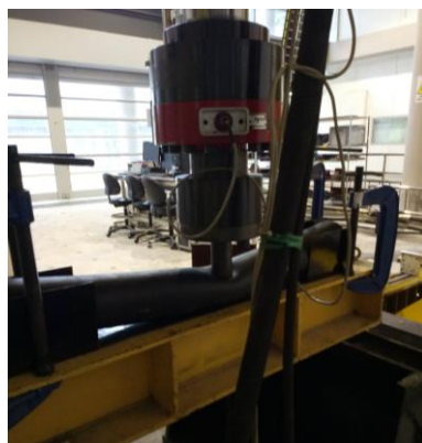
Fig. 9 - Process of applying quasi-static lateral load on RTP specimen.
