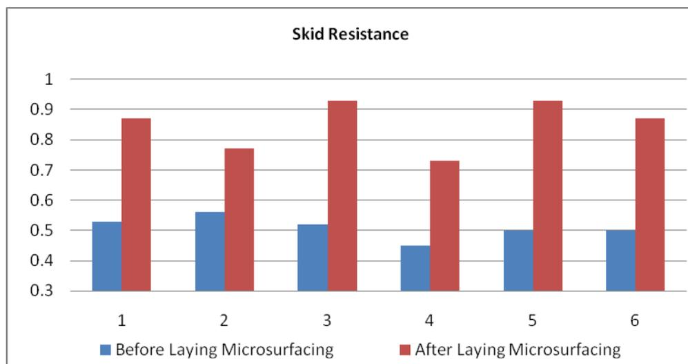
**Figure 2:** Graphical Results of Improved skid resistance
