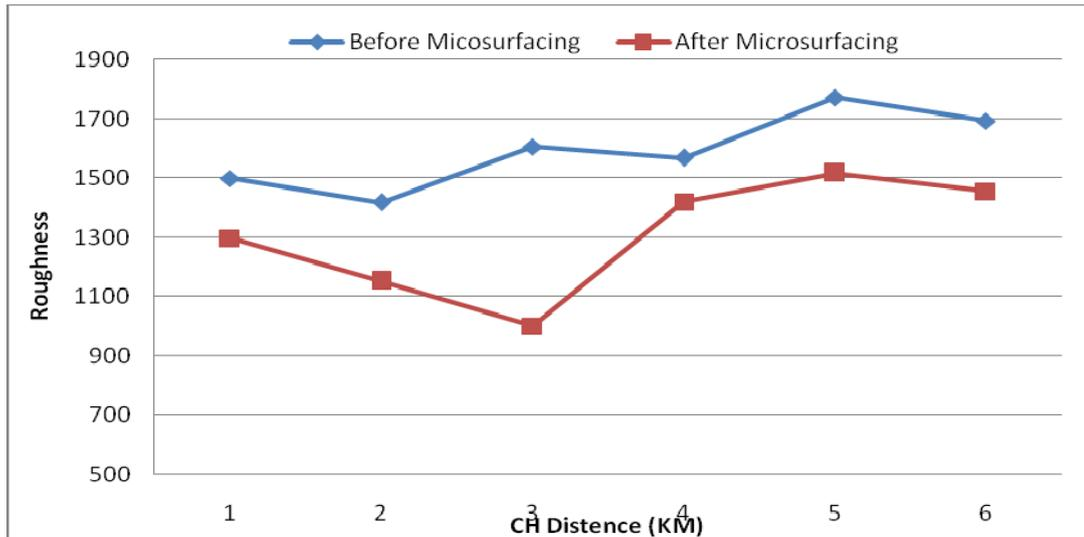
**Figure 3:** Graphical Results of Roughness
