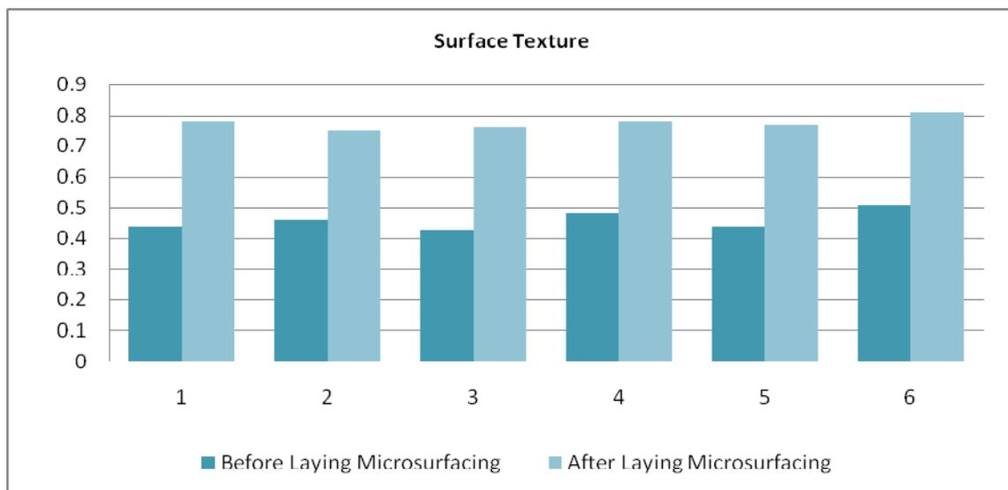
**Figure 4:** Graphical Results of Improved Surface Texture
