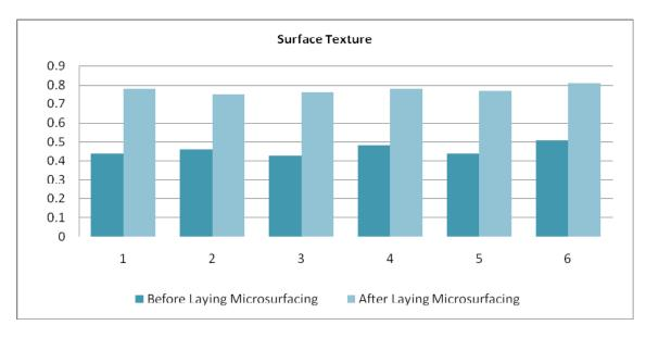
Figure 4: Graphical Results of Improved Surface Texture
