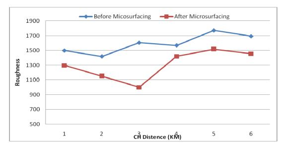
Figure 3: Graphical Results of Roughness
