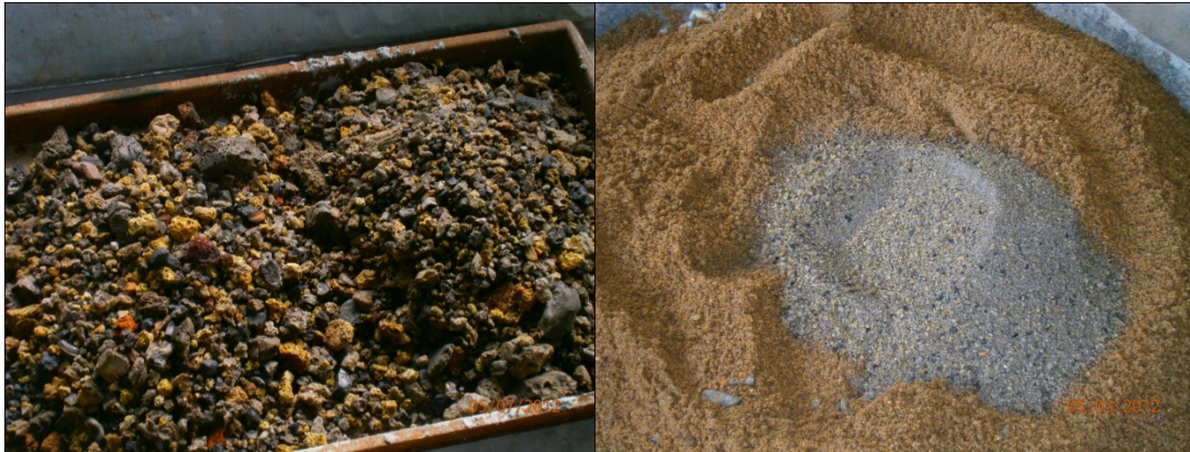
Figure 2(a) coarse bottom ash sample 5mm and above. Figure 2(b) fine bottom ash sample on fine sand passing 5mm sieve size.
