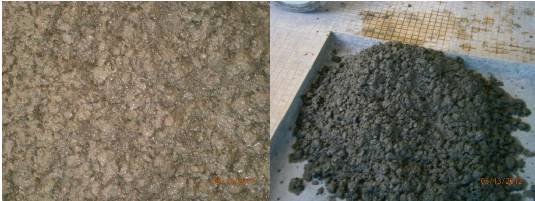
Figure 3 (a) workable CBA/FA mix Figure 3 (b) CBA/FA mix at high percentage replacement ratio.
