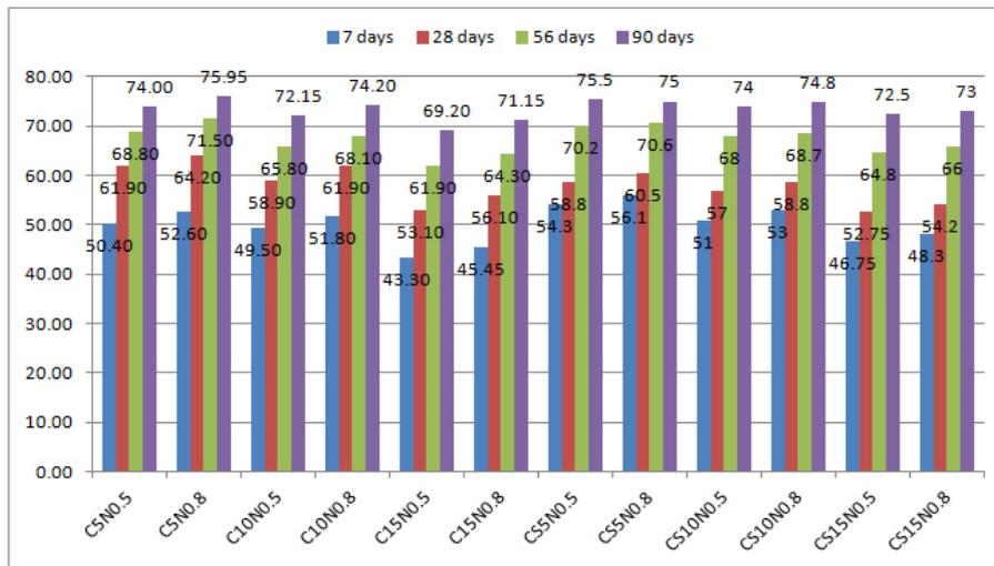
Fig. 5 - Compressive strength, (Mpa), part B
