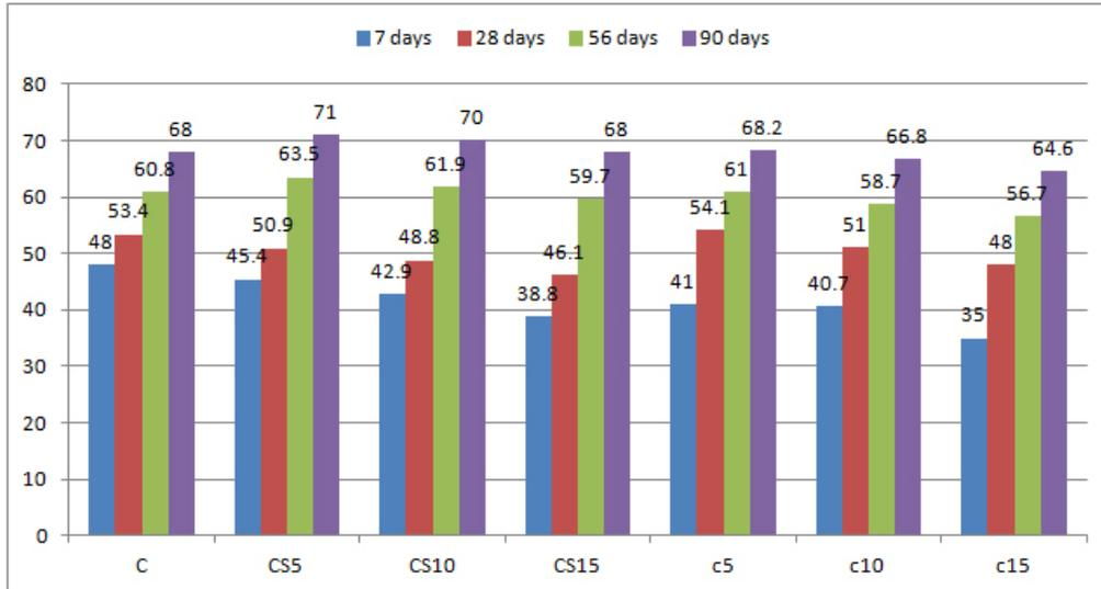
**Fig. 3 - Compressive strength (Mpa), (part A)**
