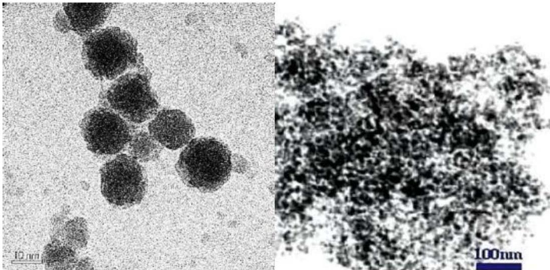
**Fig. 2 - The SEM and TEM Analysis of Nano-silica**
