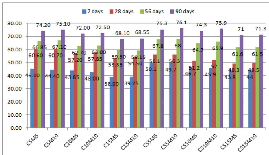
Fig. 6 - Compressive strength, (Mpa), part B
