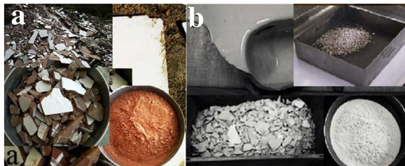
**Fig. 1 - Ceramic waste powder preparation process**
