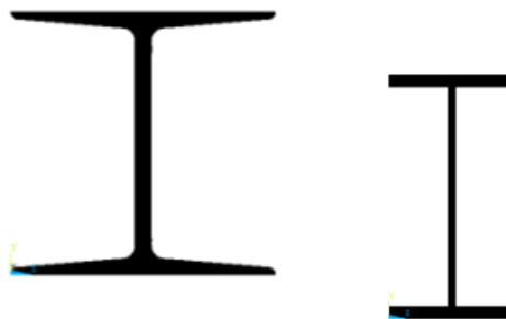
Figure 1: A) Hot rolled tapered flange I section, B) Hot rolled parallel flange I section
