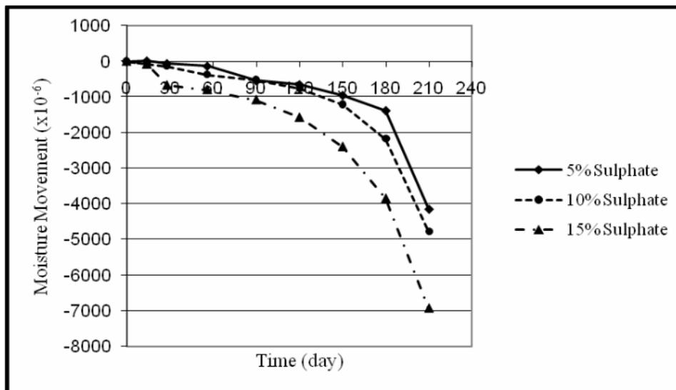
**Figure 10:** Horizontal moisture movement of fired clay masonry wall exposed to sodium sulphate
