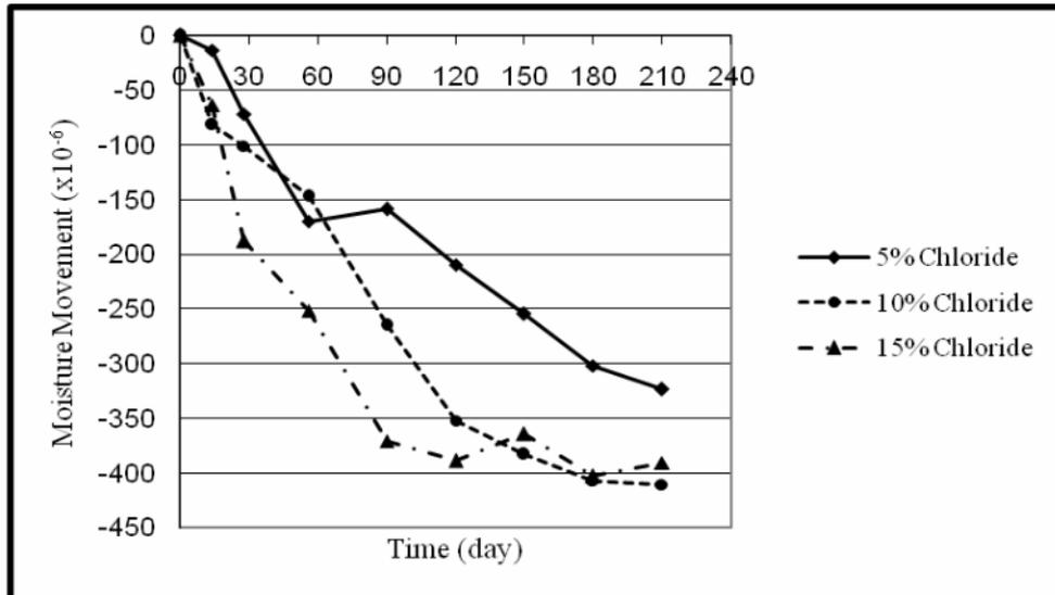
**Figure 6:** Moisture movement of fired clay brick exposed to sodium chloride
