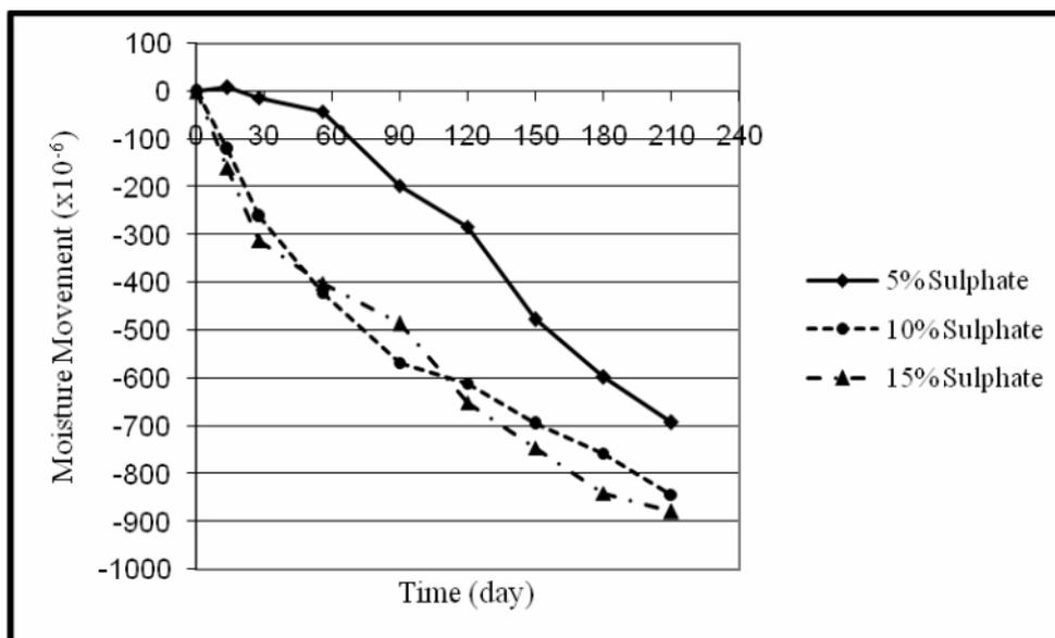
**Figure 5:** Moisture movement of fired clay brick exposed to sodium sulphate
