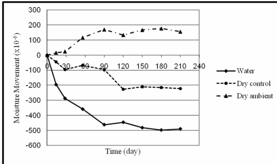
**Figure 8:** Horizontal moisture movement of control fired clay masonry wall
