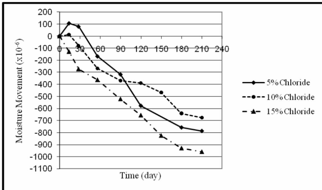
**Figure 12:** Vertical moisture movement of fired clay masonry wall exposed to sodium chloride
