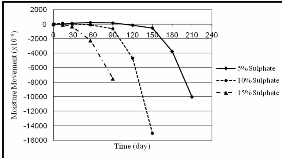
**Figure 2:** Moisture movement of mortar prism exposed to sodium sulphate
