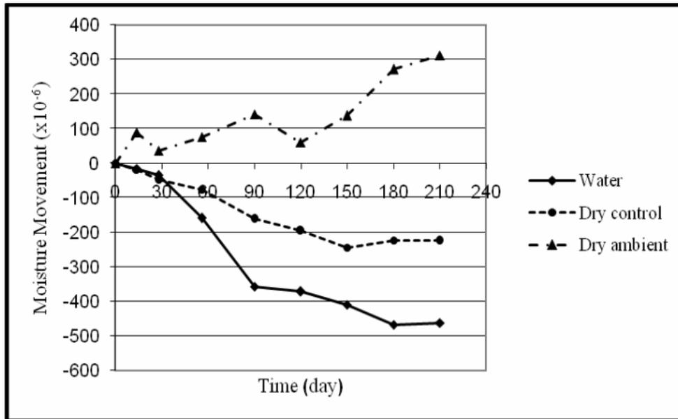
**Figure 4:** Moisture movement of control fired clay bricks
