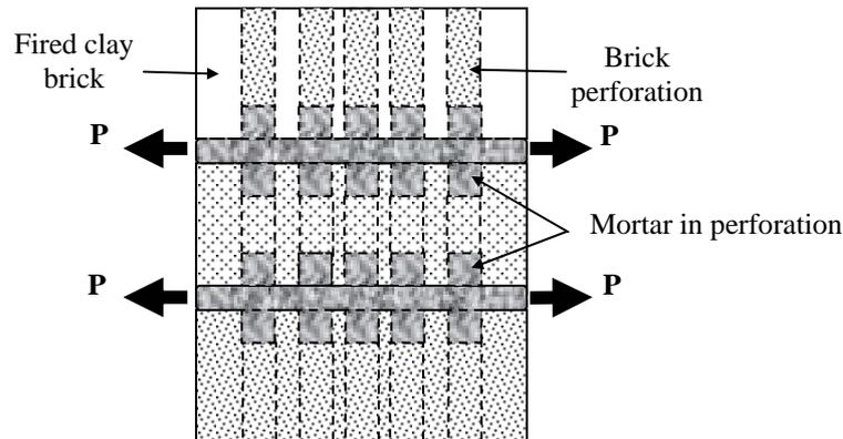
**Figure 11:** The fired-clay brickwork subjected to bonded brick-mortar restraint
