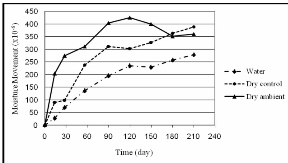
Figure 1: Moisture movement of control mortar prism
