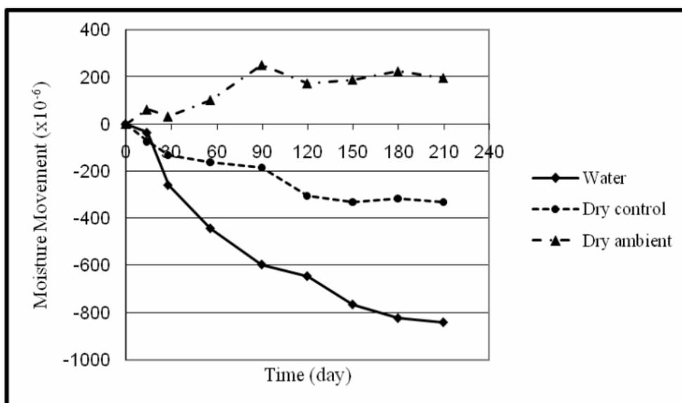
**Figure 7:** Vertical moisture movement of control fired clay masonry wall
