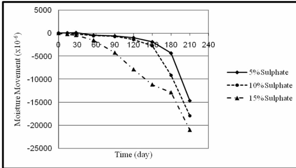
**Figure 9:** Vertical moisture movement of fired clay masonry wall exposed to sodium sulphate
