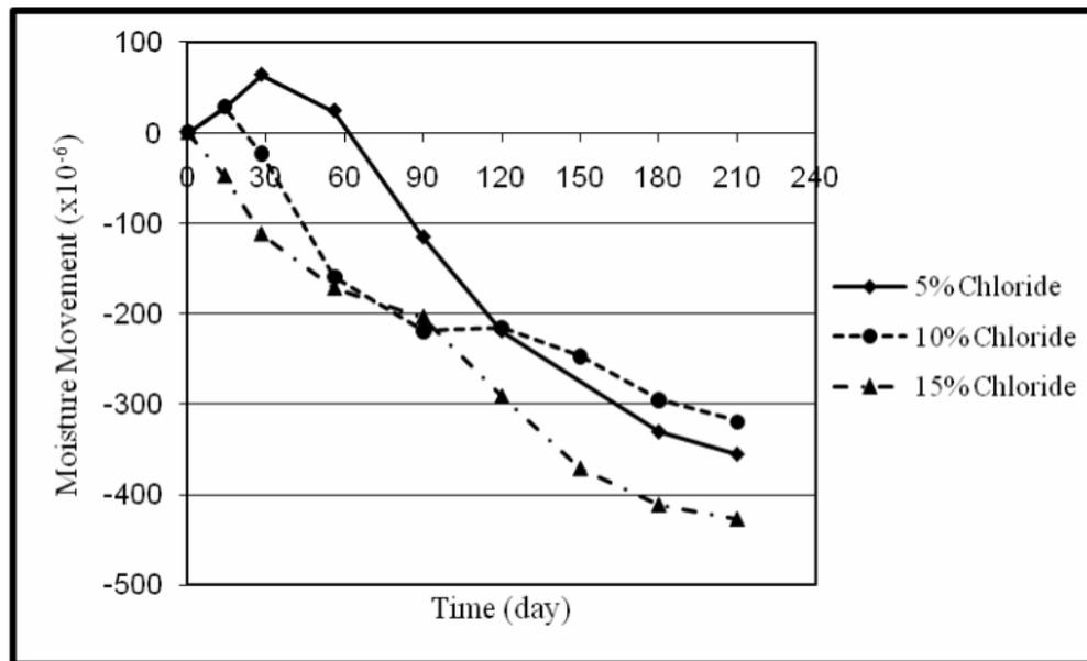
**Figure 13:** Horizontal moisture movement of fired clay masonry wall exposed to sodium chloride
