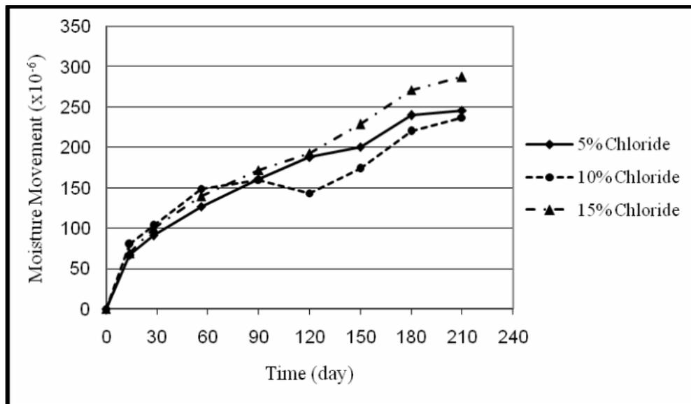
**Figure 3:** Moisture movement of mortar prism exposed to sodium chloride
