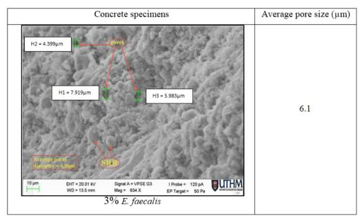
Fig. 10 - Concrete sample with *E. faecalis*
