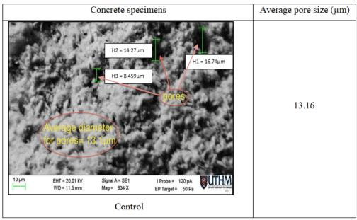
**Fig. 9 - Microstructure of normal concrete**
