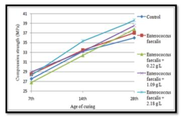
Fig. 5 - Compressive Strength of bio-concrete and calcium lactate
