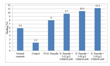
Fig. 8 - Percentage of healing for crack by 3-point bending
