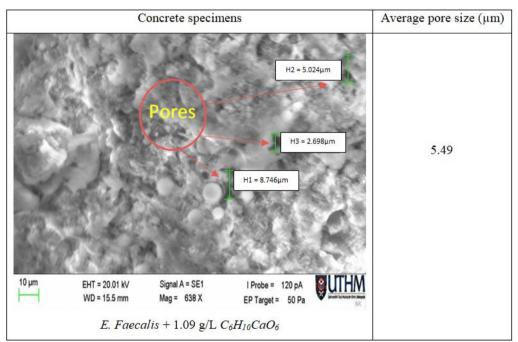
Fig. 12 - Concrete sample with E. Faecalis and 1.09g/L calcium lactate
