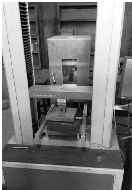
Figure 1: Brick in the Testometric machine
