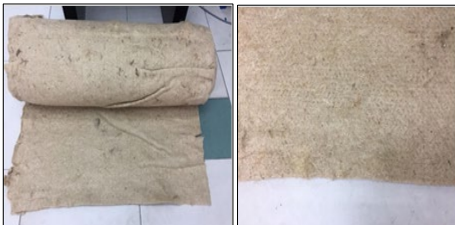
Fig. 2 Physical appearance of Kenaf Fiber (KF) chopped strand mat
