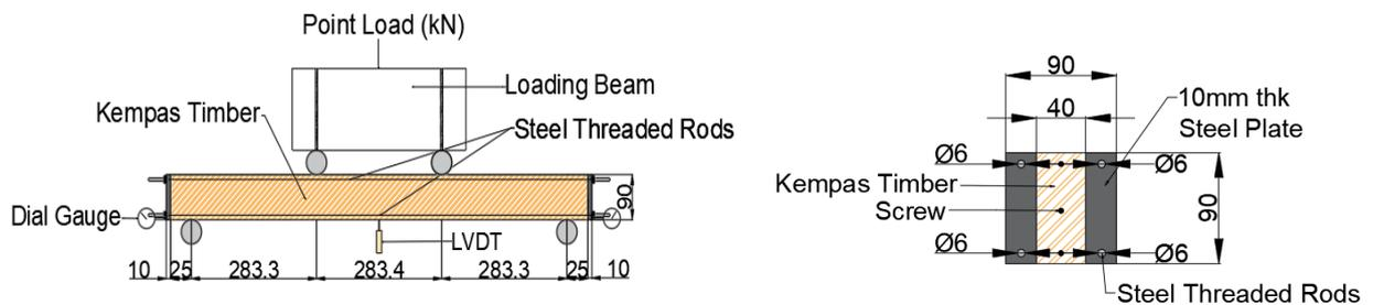
**Fig. 8 - Four-point bending test setup (left) and cross-section (right) for TBTC specimen type (dimensions in mm)**
