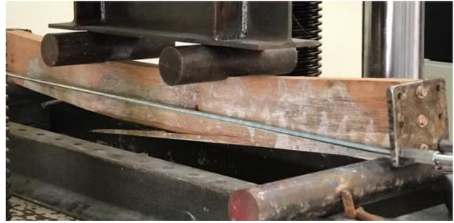
**Fig. 12 - Typical split tension failure at lower fibre tension zone of timber beam with passive prestressing**
