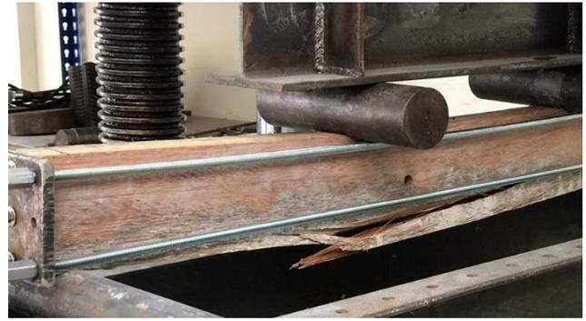
**Fig. 14 - Typical split tension failure at lower fibre tension zone of timber beam with passive prestressing top and bottom timber fibre**
