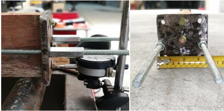
**Fig. 9 - Anchorage 10 mm steel plate and prestress threaded rods fastened with long nuts**
