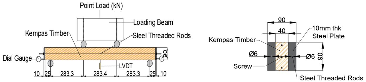
**Fig. 5 - Four-point bending test setup (left) and cross-section (right) for TBN specimen type (dimensions in mm)**
