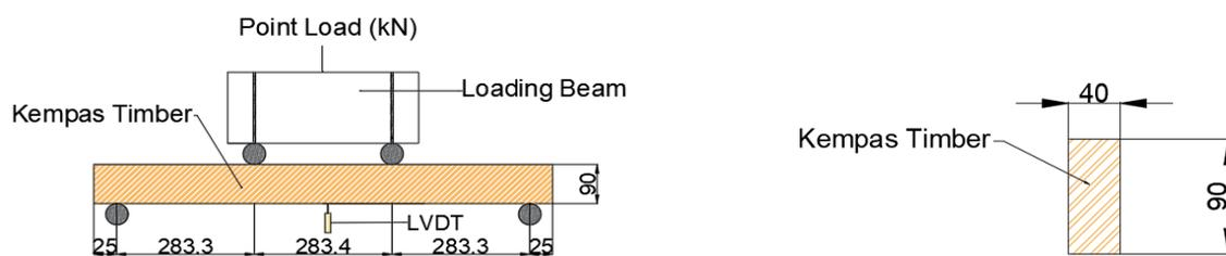
**Fig. 4 - Four-point bending test setup (left) and cross-section (right) for TB specimen type (dimensions in mm)**
