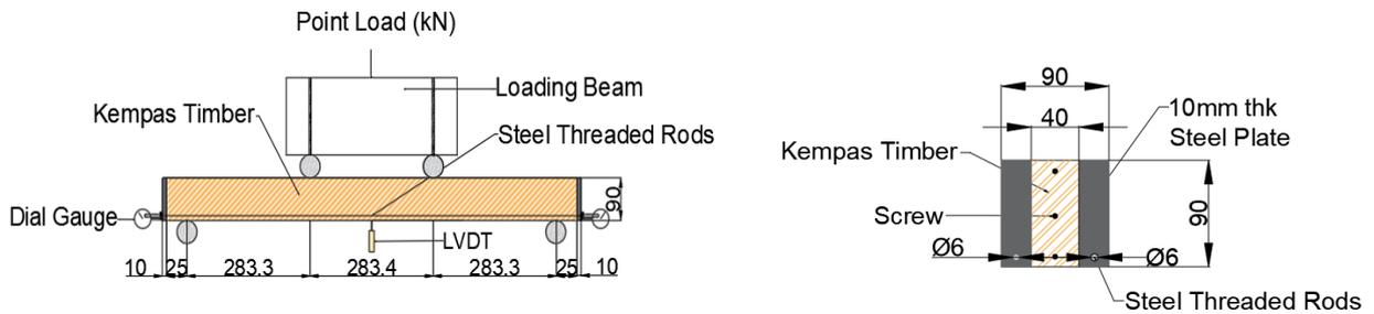
**Fig. 7 - Four-point bending test setup (left) and cross-section (right) for TBT specimen type (dimensions in mm)**
