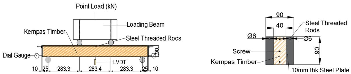
**Fig. 6 - Four-point bending test setup (left) and cross-section (right) for TBC specimen type (dimensions in mm)**
