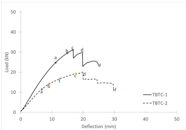
**Fig. 19 - Four-point bending load-deflection graph for TBTC specimen**
