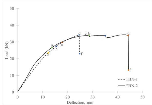
**Fig. 16 - Four-point bending load-deflection graph for TBN specimen**
