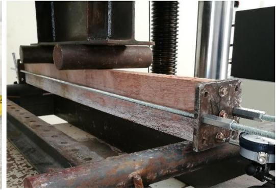
**Fig. 10 - Typical experimental setup of four-point bending test**
