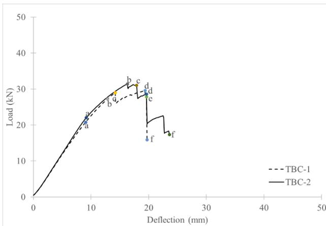
**Fig. 17 - Four-point bending load-deflection graph for TBC specimen**
