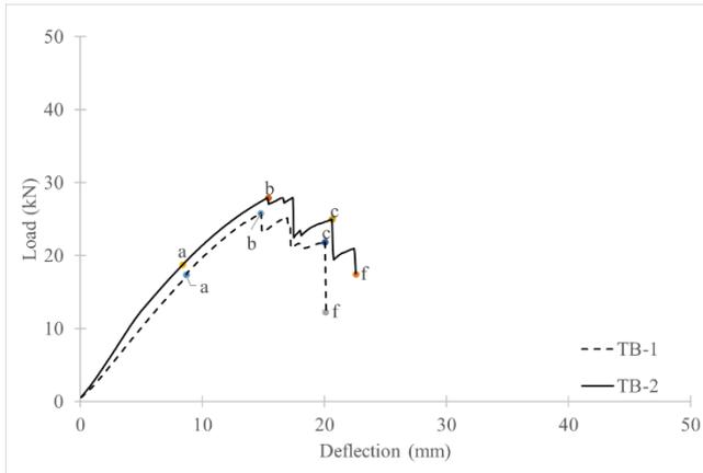
**Fig. 15 - Four-point bending load-deflection graph for TB specimen**
