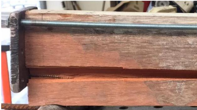
**Fig. 13 - Compression parallel to grain failure of timber at anchorage end plate**
