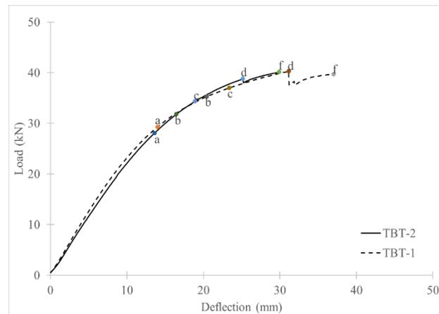
**Fig. 18 - Four-point bending load-deflection graph for TBT specimen**
