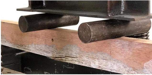
**Fig. 11 - Typical split tension failure at lower fibre tension zone of timber beam without prestressing**
