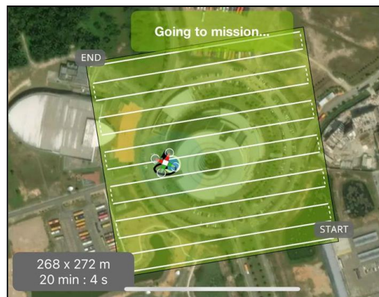
Fig. 3 - Planned flight path from plan view in grid motion
