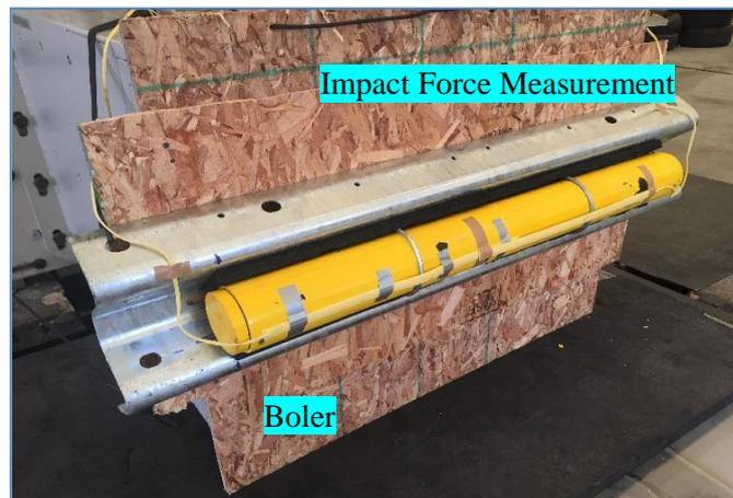
Figure 6 : The specimen was mounted on the rigid offset barrier block
