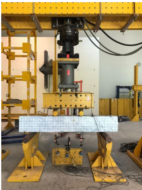
Fig. 2 4 Point Load Test of RC Beam Specimens
