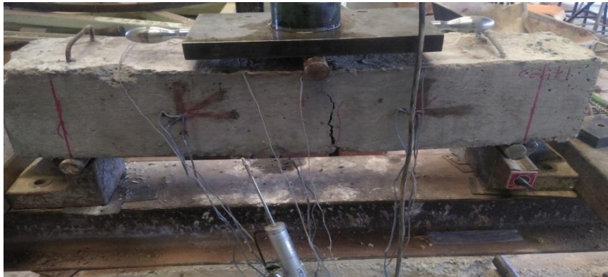
Fig. 8 Test of the Beam under Three-Point Load
