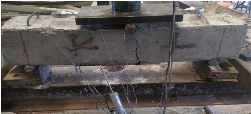
Fig. 6 Simply supported beam subjected to three points load
