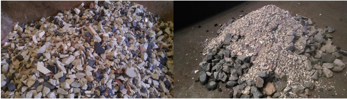
Fig. 1 Fine and coarse waste glass and ceramic tiles
