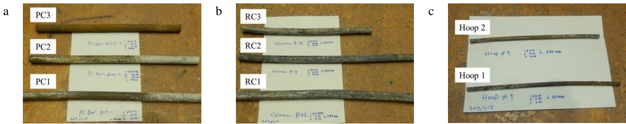
Fig. 7 - Samples of (a) PC steel rods; (b) column RC bars; (c) shear reinforcement
