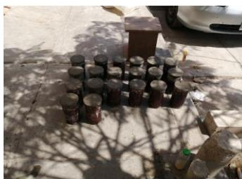
**Fig. 5** Emptying specimens NTP 339.034
