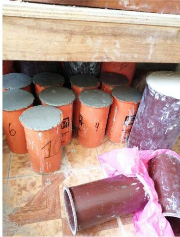
**Fig. 7** Filling of test specimens for testing NTP 339.084
