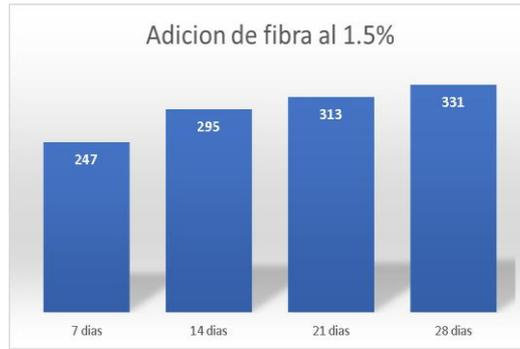
**Fig. 11** Graph of the values obtained by Resistance to 1.5%
