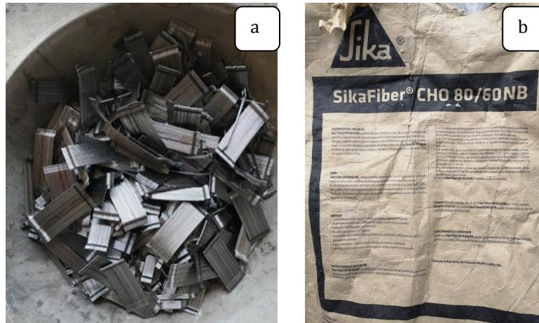
Fig. 3 (a) Wire fibres; (b) Sika Fiber bag CHO 80/60 NB
