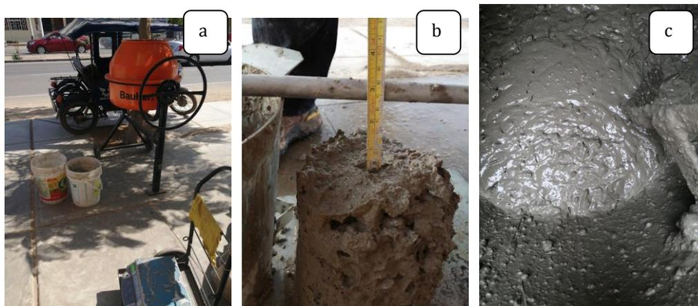
**Fig. 4** (a) Elements used for concrete preparation, (b) Slump measurement, (c) Concrete mixed with fiber additions
