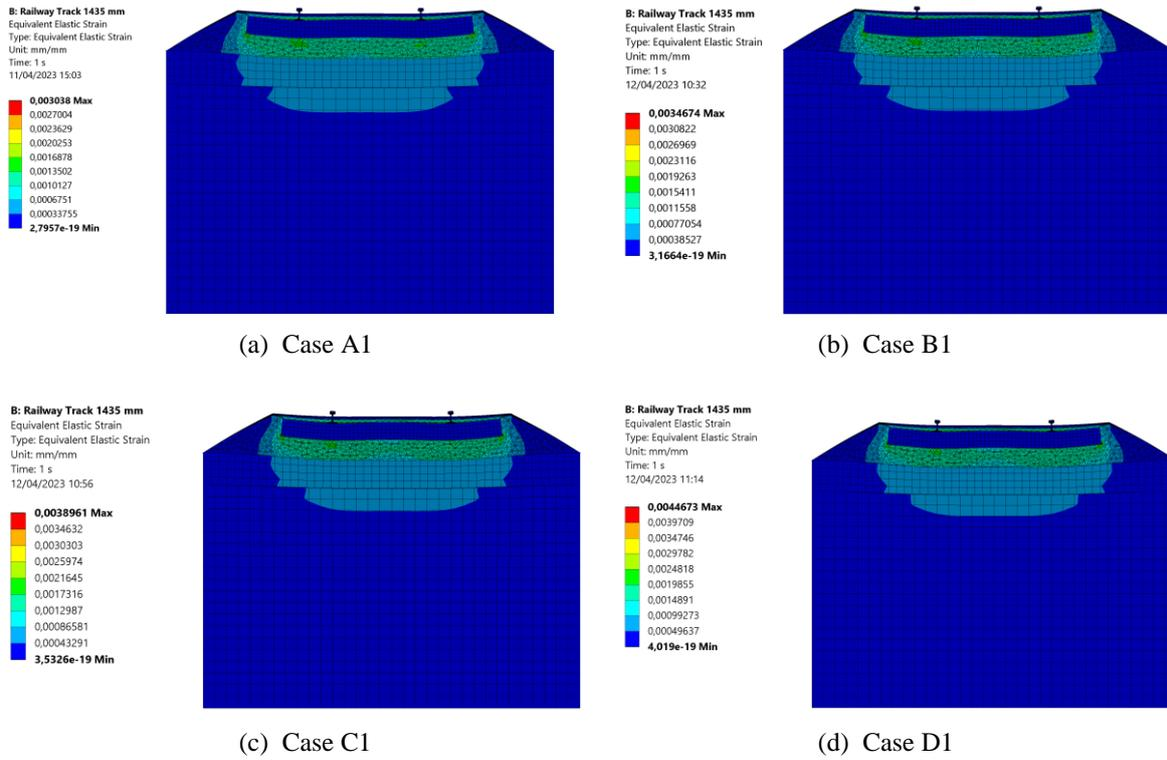
**Fig. 12 - Strain Distribution of 1435 mm Gauge**
