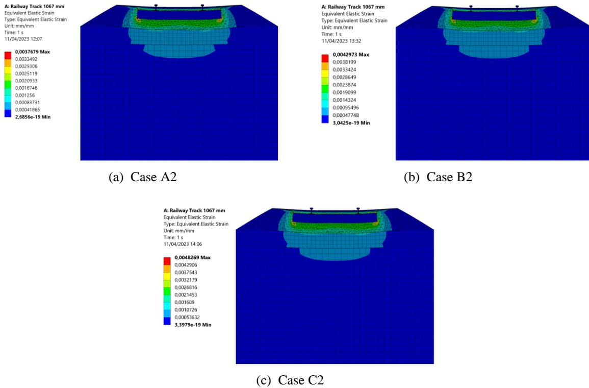
**Fig. 13 - Strain Distribution of 1067 mm Gauge**
