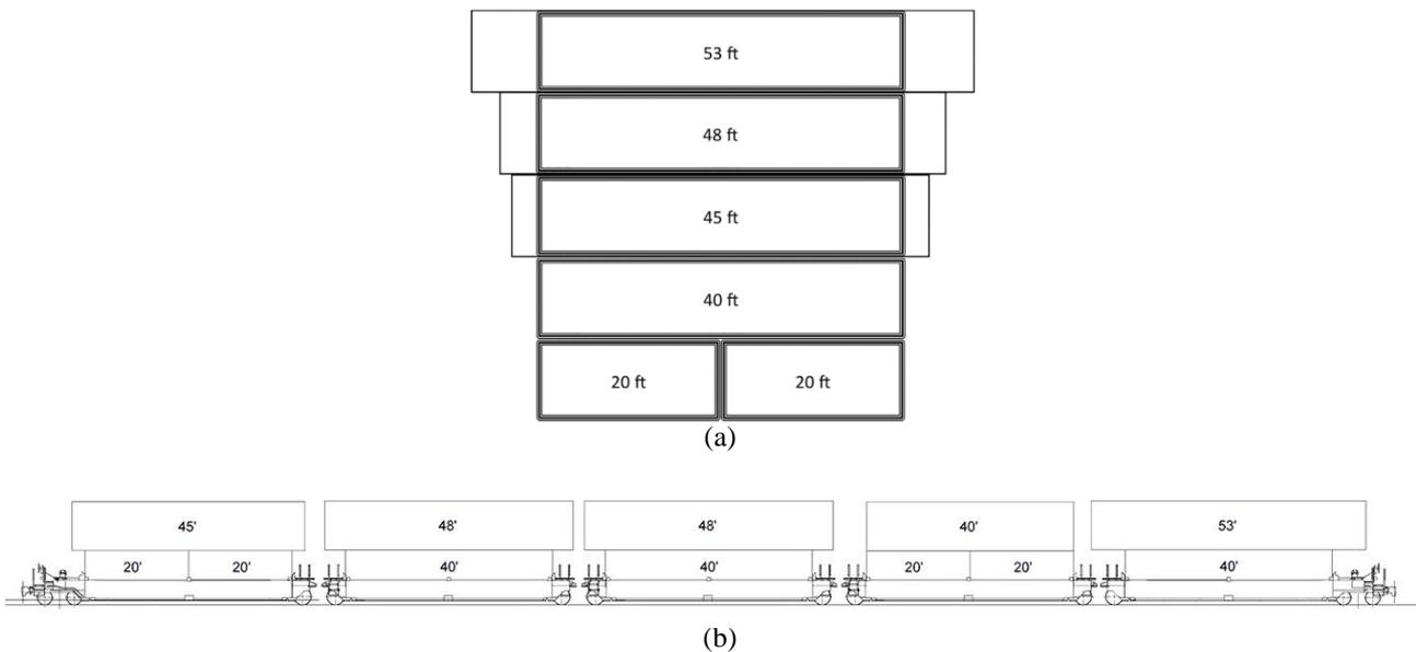
**Fig. 1 - Container Stacking Configuration in Double-Stack Freight Train: (a) Arrangement of stacking (Mantovani et al., 2018); (b) Example of stacking for different configurations in a trainset (www.gbrx.com, 2022)**
