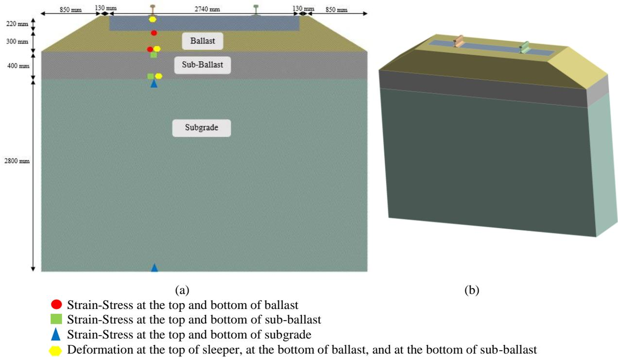
**Fig. 4 - Dimension Model of 1435 mm Gauge Railway Track: (a) Cross Section Model Dimension and Measuring Point; (b) 3D Model for Analysis**
