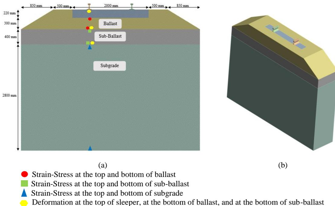
**Fig. 3 - Dimension Model of 1067 mm Gauge Railway Track: (a) Cross Section Model Dimension and Measuring Point; (b) 3D Model for Analysis**
