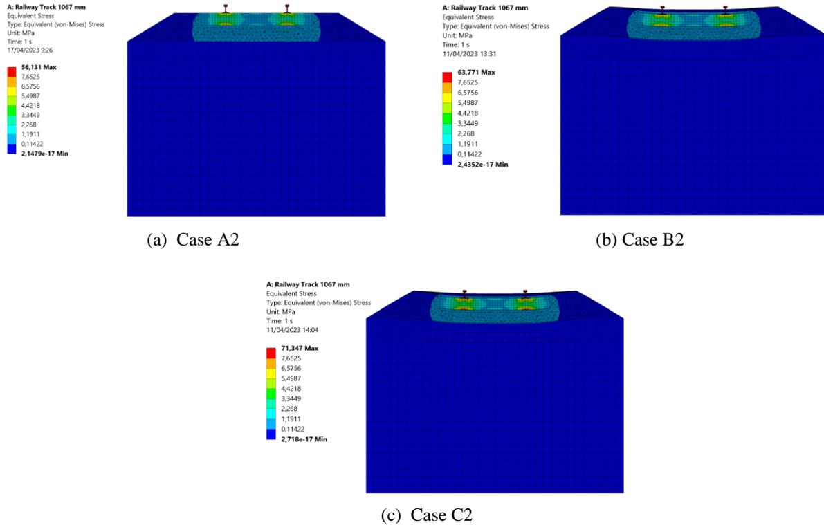
**Fig. 10 - Stress Distribution of 1067 mm Gauge Track**
