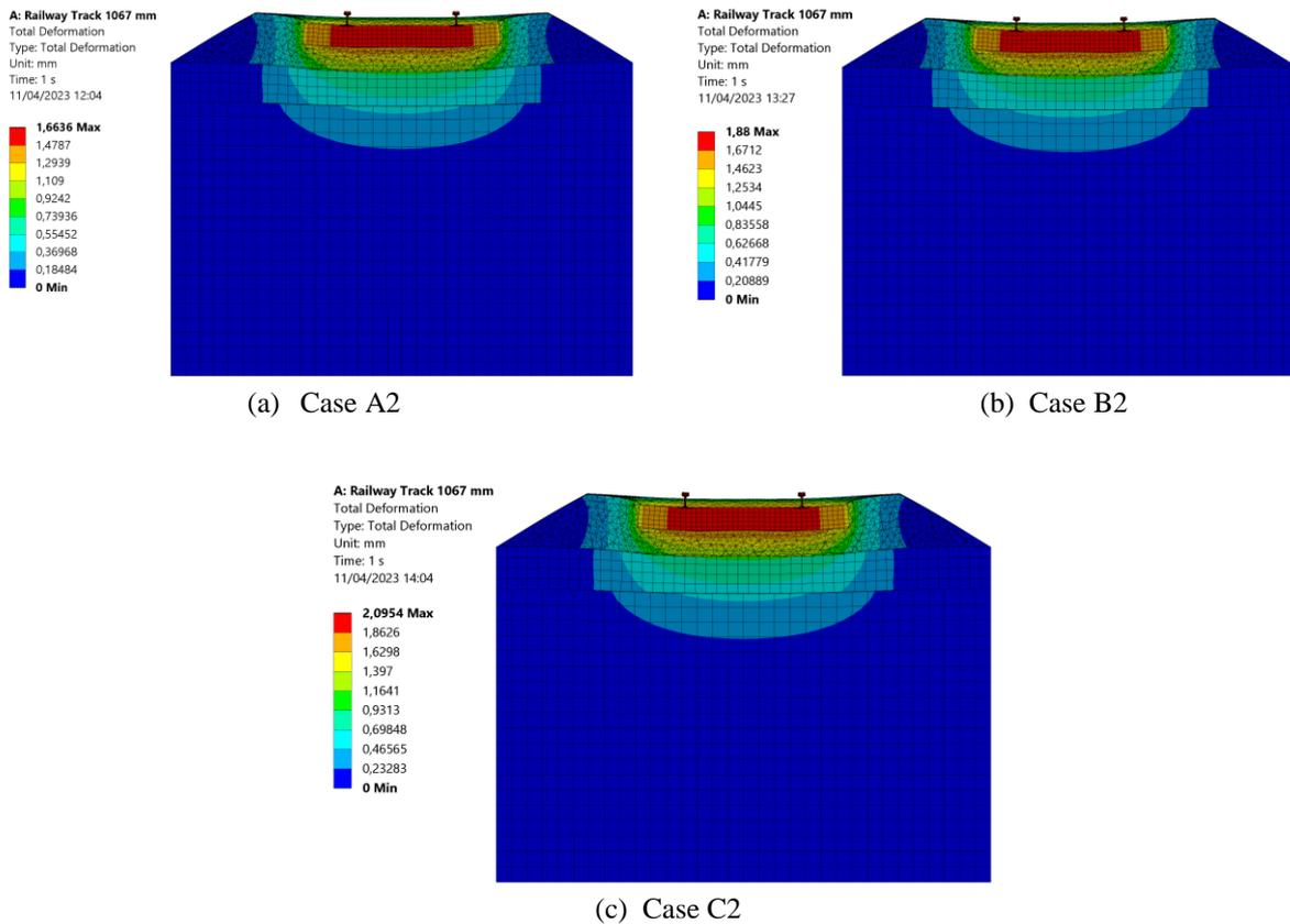
**Fig. 7 – Deformation Distribution of 1067 mm Gauge Track**
