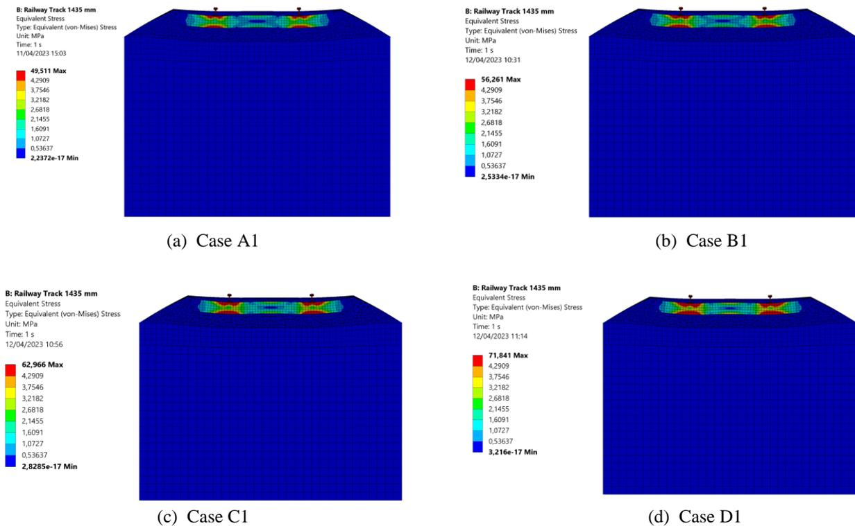
Fig. 9 - Stress Distribution of 1435 mm Gauge Track
