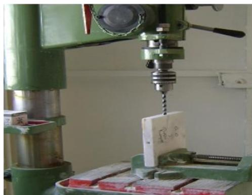
**Fig. 1 - Drilling the dowel hole**
