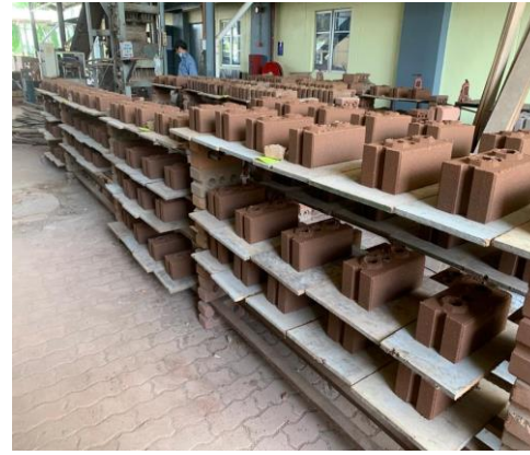
Fig. 5 - CEBs undergo dry curing for 7 days and 28 days
