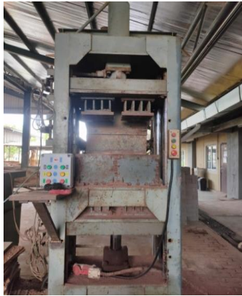
Fig. 4 - Compressed stabilized earth block machine
