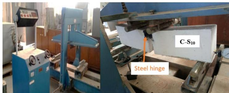
**Fig. 3 - Testing Set-up of the Beam Specimen under test machine**
