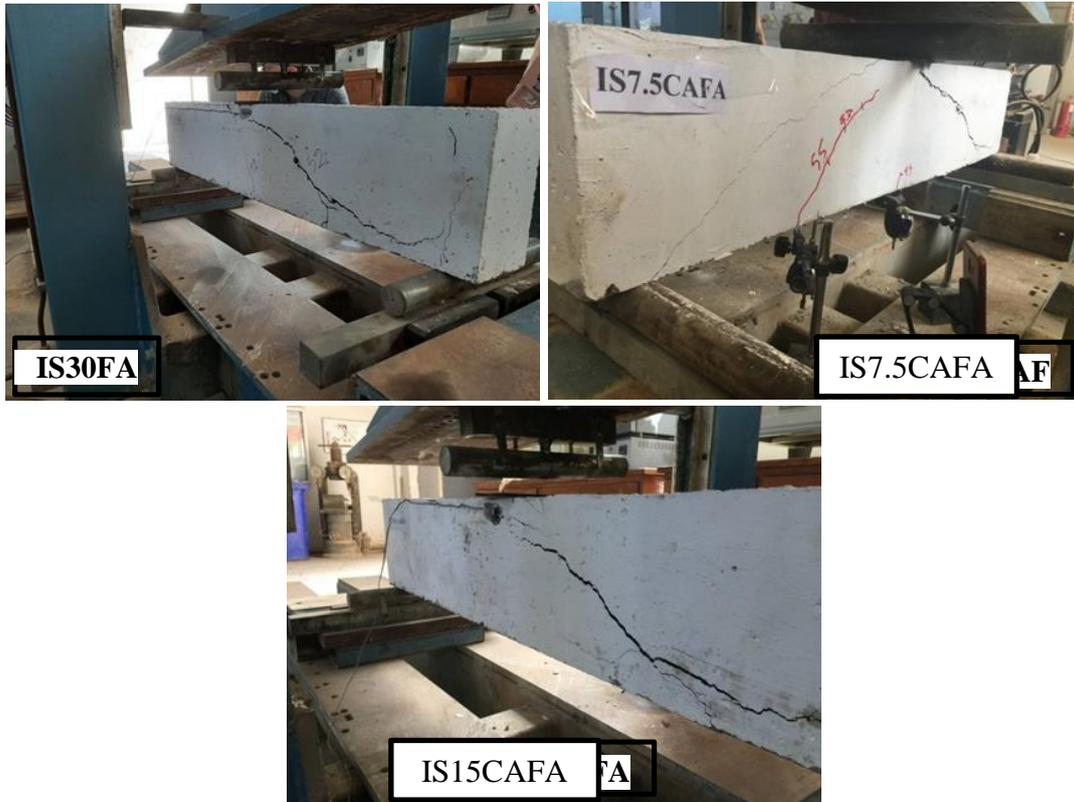
Fig. 7 - Failure mode of tested beams
