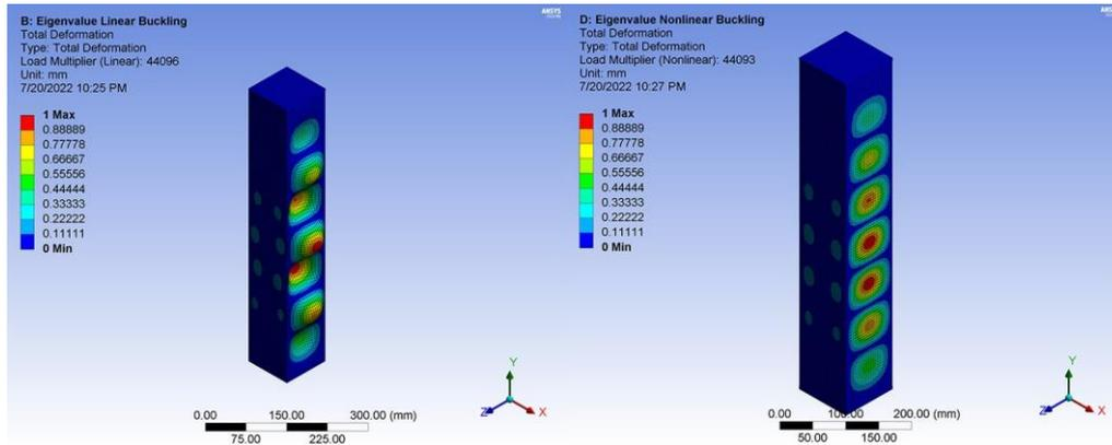
(i) Pre-stress linear and non linear buckling of AS1
