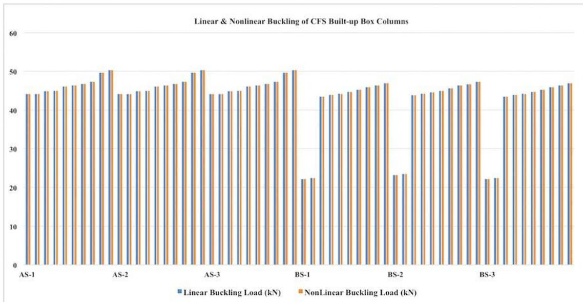
Fig. 5 - Comparison of linear and non linear buckling of Group A & B
