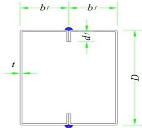
**Fig. 1 - Parameters of typical tested specimens**
