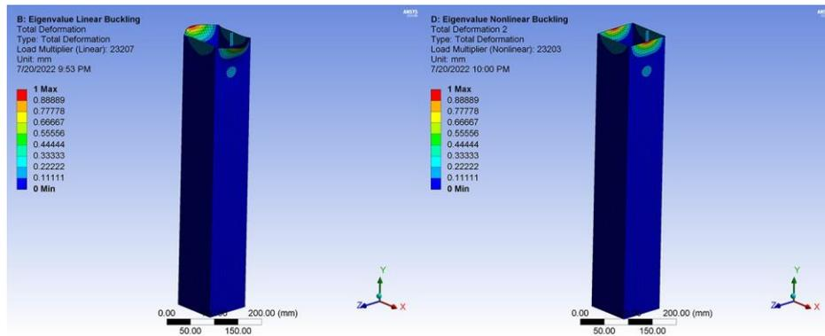
(ii) Pre-stress linear and non linear buckling of BS2
