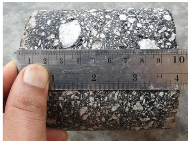
Fig. 4 - The cored asphalt sample showing a 10 cm in thickness
