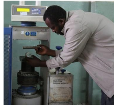
Fig. 1 - Loading on the specimen and testing for split tensile strength
