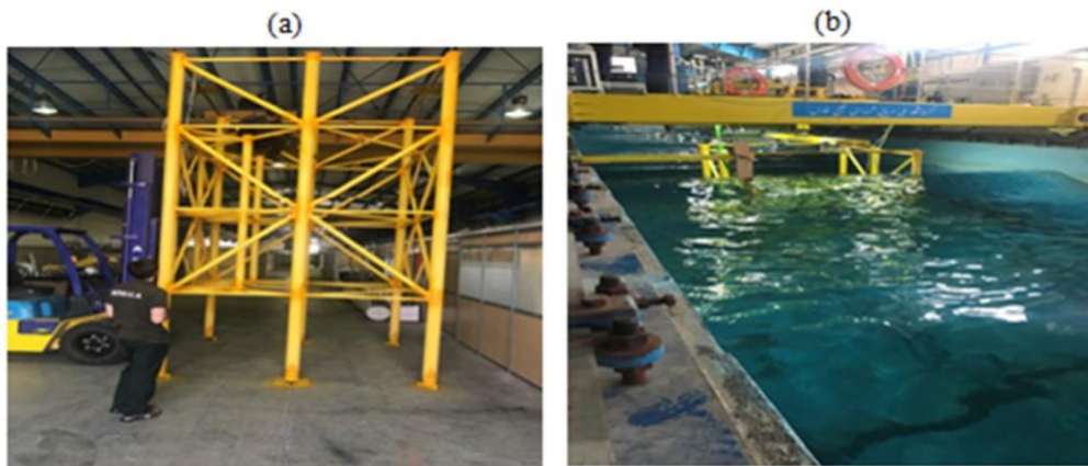
Fig. 4 - (a) Dry jacket structure; (b) the jacket installed in the flume without the wave barrier
