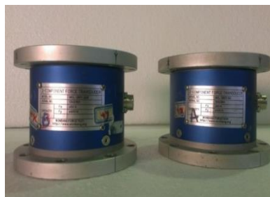
Fig. 5 - Load cells used in the present research to measure the wave forces
