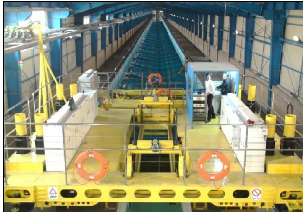
Fig. 1 - The wave flume and manned chariot of NIMALA marine laboratory
