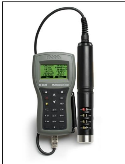
Fig. 6 - The multi-parameter to measure the pH, temperature and dissolved oxygen
