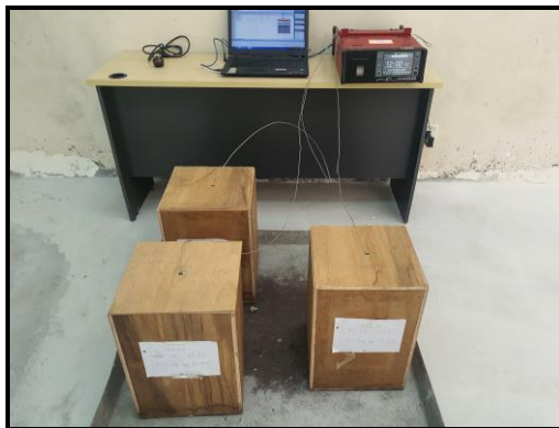
Fig. 4 - Hydration temperature of concrete testing equipment
