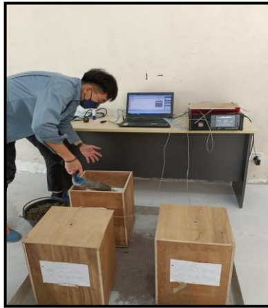
Fig. 2 - Pouring concrete into mould
