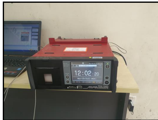
Fig. 5 - System for recording temperature data via a data logger
