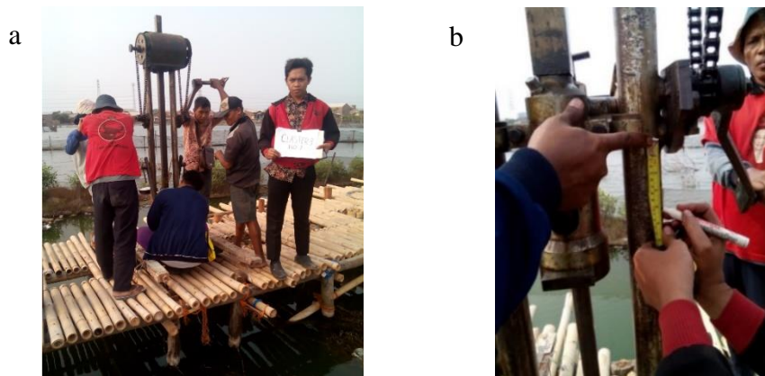
Fig. 10 - Cluster test (a) cluster load test; (b) cluster displacement reading
