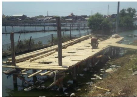
Fig. 7 - The platform of the cluster load test
