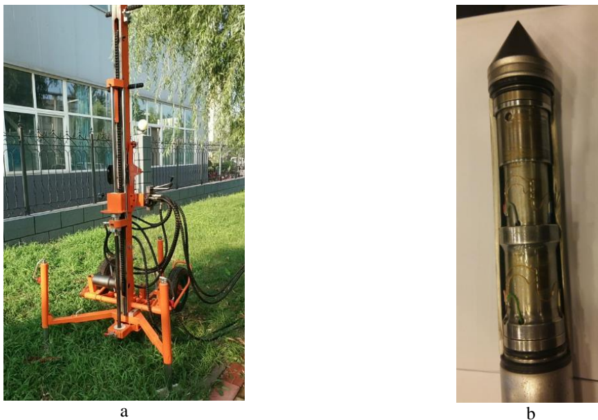
Fig. 2 - (a) Test Soil bearing capacity Multifunction Standard Penetration Test and Dynamic Cone Penetrometer and; (b) CPT Apparatus
