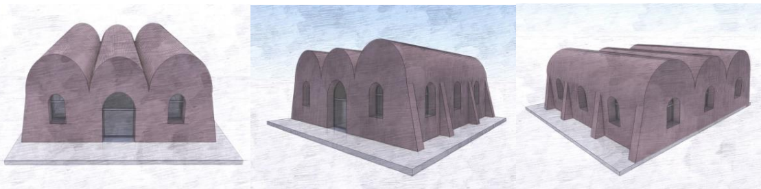
Fig. 1 - Perspective of the model showing the structure generated from the arched frames
