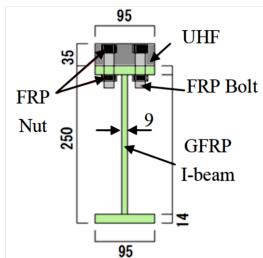
Figure 2: Cross-section of UHFGFRP I-beam (mm) [27]
