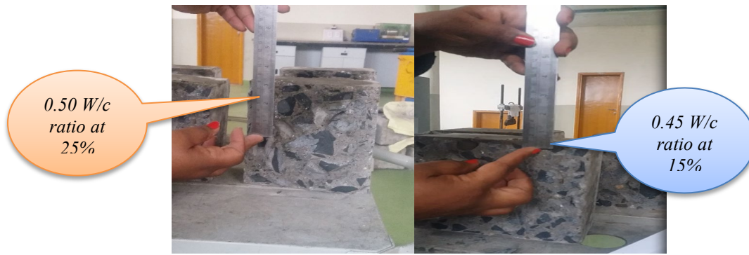
Fig. 8 - Cube specimens testing for concrete permeability test
