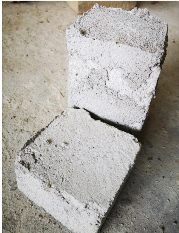
Fig. 7 - Failure pattern detected during shear tests
