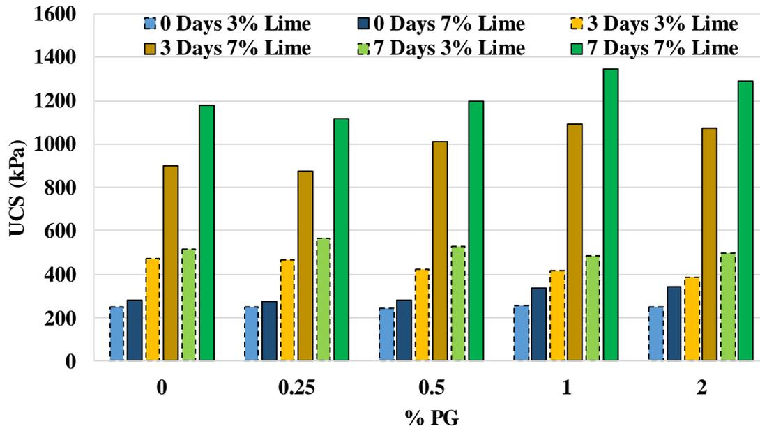
Figure 3: Strength of Lime Stabilized Soil with PG
