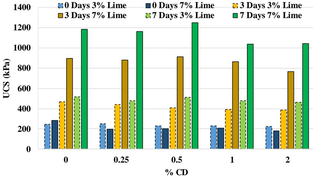
Figure 5: Strength of Lime Stabilized Soil with CD
