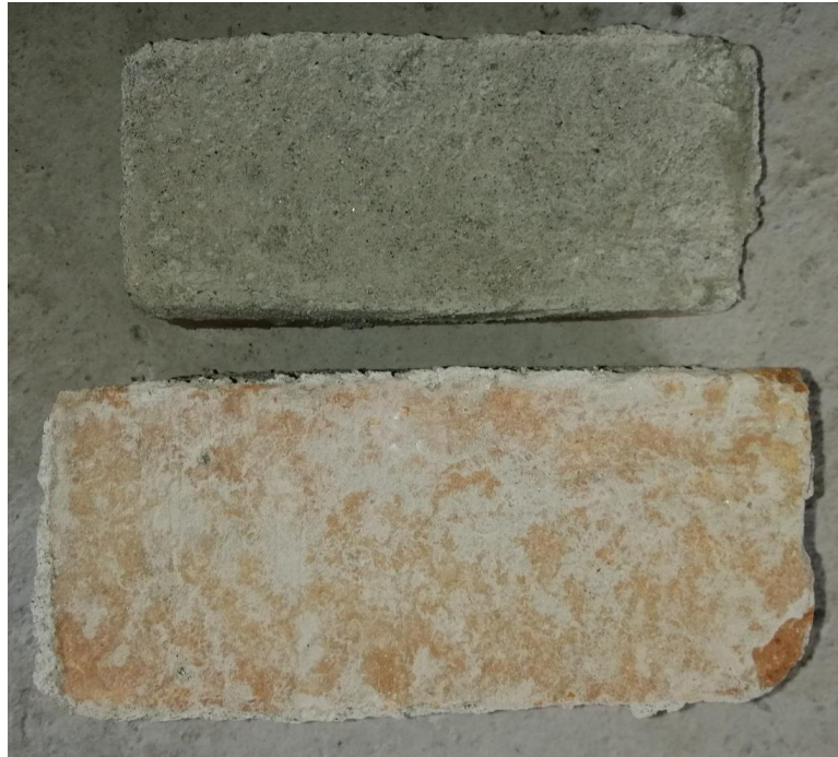
Fig. 10 - Failure pattern of the masonry triplet under shear loading
