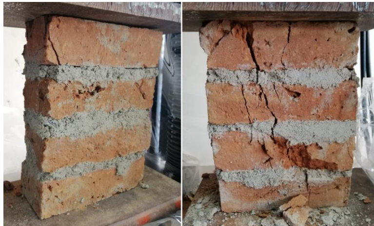
Fig. 8 - Typical compressive failure modes in masonry prisms
