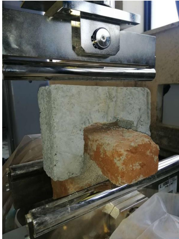
Fig. 3 - The test setup used for the measure of bond strength of masonry cross-couplet
