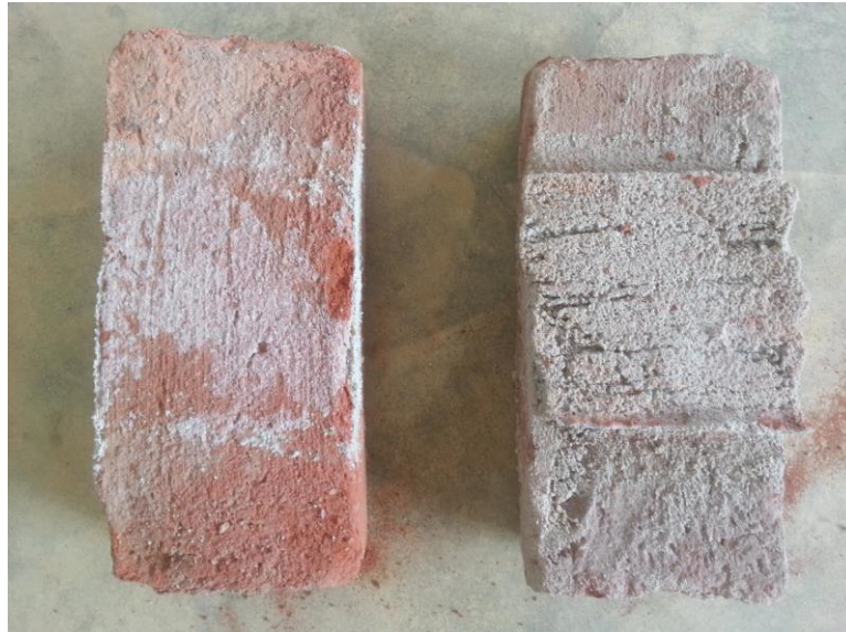
Fig. 12 - The failure pattern observed in the bond test
