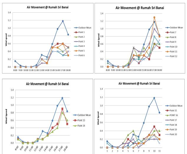
Figure 12: Graph of Wind Speed against Time for Sri Banai House
