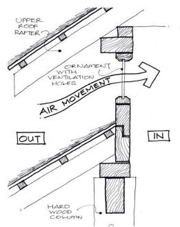
Figure 14: Air Movement Flow between Roofs
