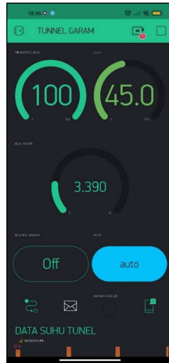
Figure 7 (b): Heater auto control display
