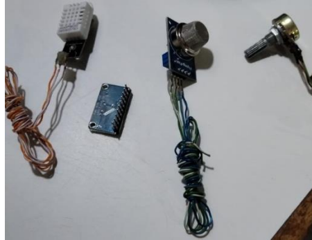
Figure 3: Sensors and analog-digital converter
