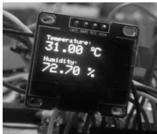
Figure 7: The temperature and humidity reading displayed on OLED I2C
