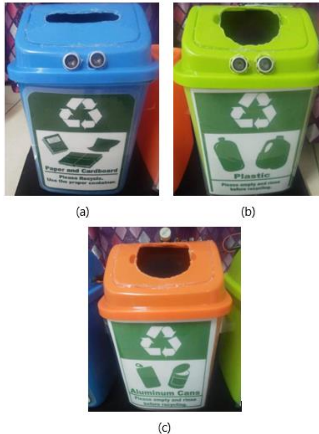
Figure 7: Prototype of (a) paper recycle bin; (b) plastic recycle bin and; (c) aluminium can recycle bin
