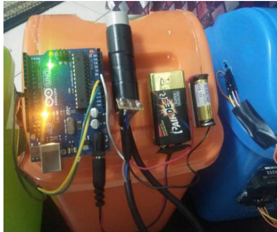
Figure 11: Circuit of inductive proximity sensor and servo motor for aluminium recycle bin
