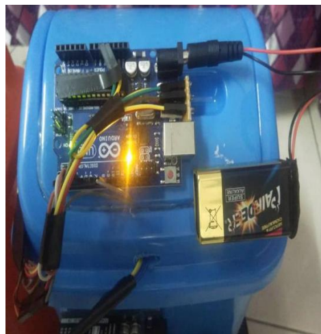
Figure 10: Circuit of ultrasonic sensor and servo motor for paper recycle bin
